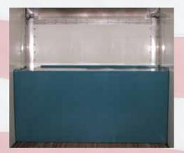
The water tank is designed to help maximize space in your truck while keeping the water from freezing and all components warm. The 250 gallon water tank can be used for blowing stabilized insulation in the attic or in wall spray applications.
