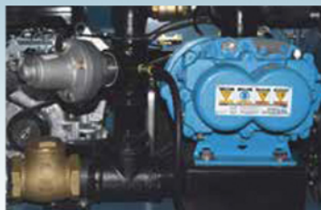
Positive Displacement Blower w/250 CFM @ 6PSI (Diesel & PTO) w/220 CFM @ 5PSI (Electric)
