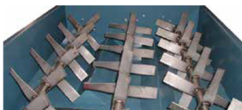
Multiple Agitators Designed for Constant Material Flow
