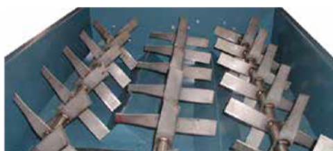
Multiple Agitators Designed for Constant Material Flow
